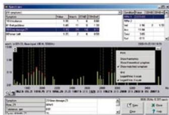
An Evam<sup>®</sup> spectrum highlights the selected fault symptoms and states their velocity value in relation to overall machine vibration.
