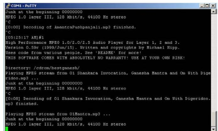
**Figure 1.** With Windows (running on another computer) and Putty you may connect to any computer (notebook) via a serial cable (serial console with KarmaBSD) and you may thus repair or control any computer
