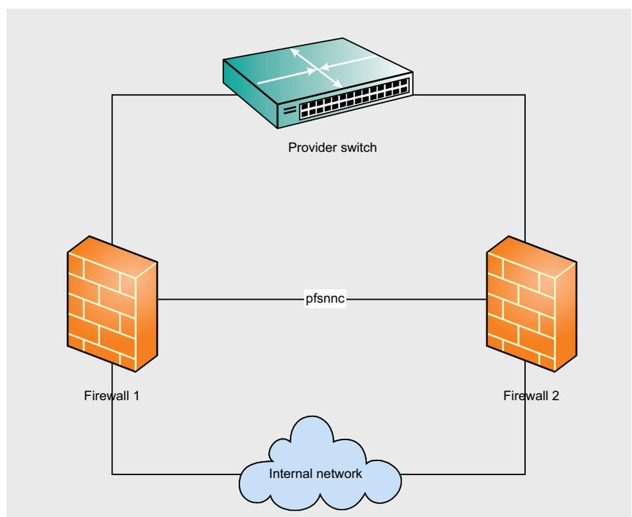
Figure 1. The illustration the basic layout of the firewall setup
