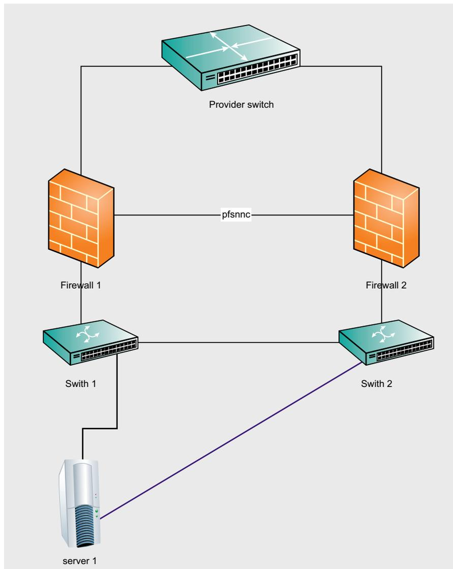
Figure 3. The illustration the above infrastructure, with server network redundancy added in
