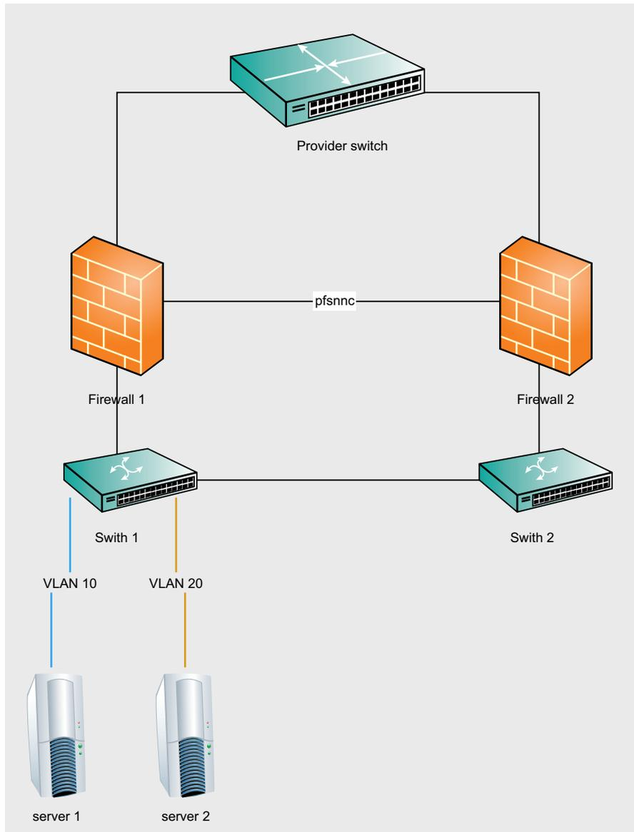
Figure 2. A firewall in networks for routing all communication between the VLANs
