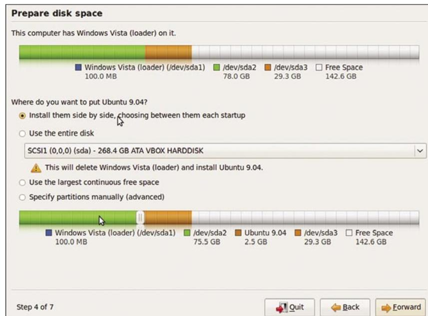
Figure 9. The partition table before installing Ubuntu
