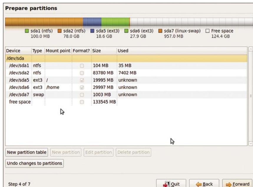
Figure 3. The partition table of a Windows- Ubuntu dual boot system...
