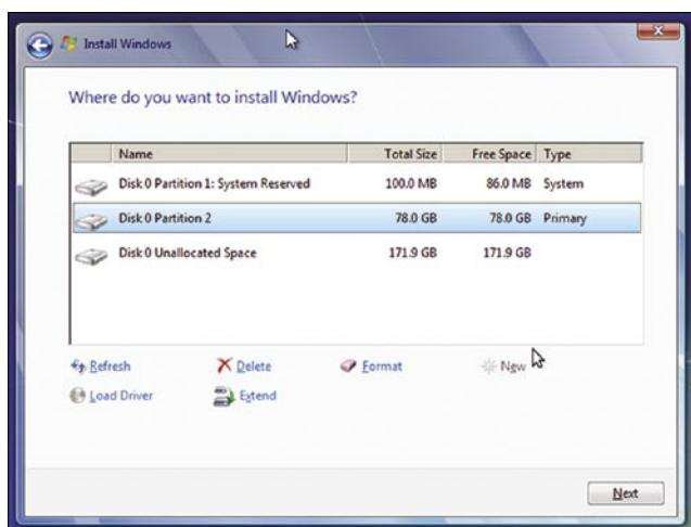
Figure 1. Windows 7 creates two primary partitions by default when installing on a blank hard drive
