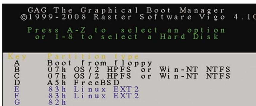
Figure 16. The partition table as recognized by GAG
