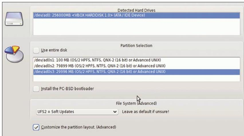
**Figure 12.** These are the proper selections for creating a working multiboot system during partitioning
