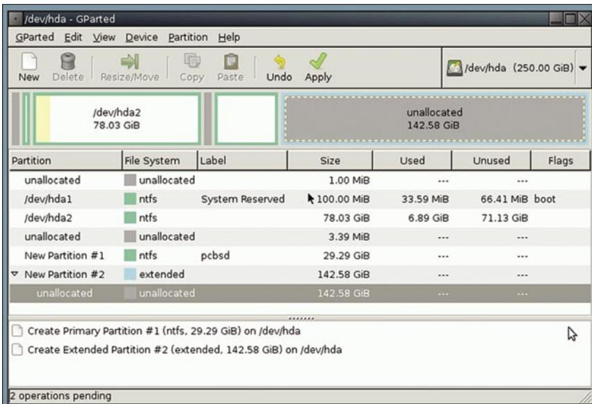
Figure 8. The new partition table as needed for installing first Ubuntu, and then PC-BSD
