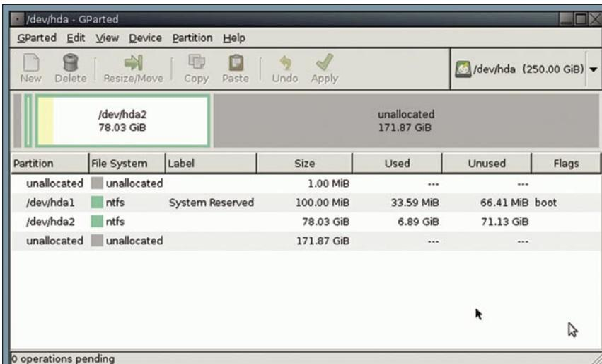
Figure 7. GParted scans the hard drive and shows the partitions used by Windows 7
