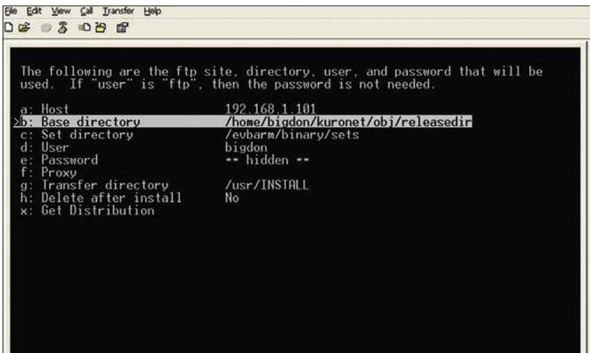
Figure 3. Setting up NetBSD to download the installation files from the local Windows machine
